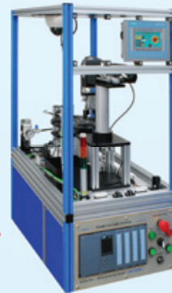
2nd test & Sorting Station (CPE-FAS30E)
